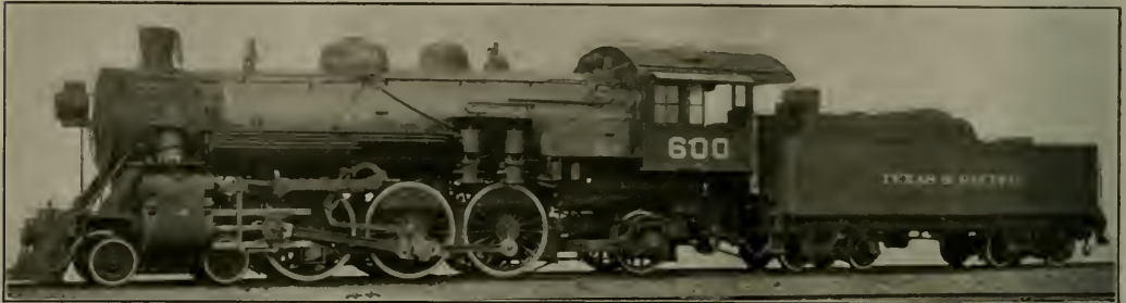
PACIFIC 4-6-2 TYPE LOCOMOTIVE FOR THE TEXAS AND PACIFIC RAILWAY, Baldwin Locomotive Works, Builders.
